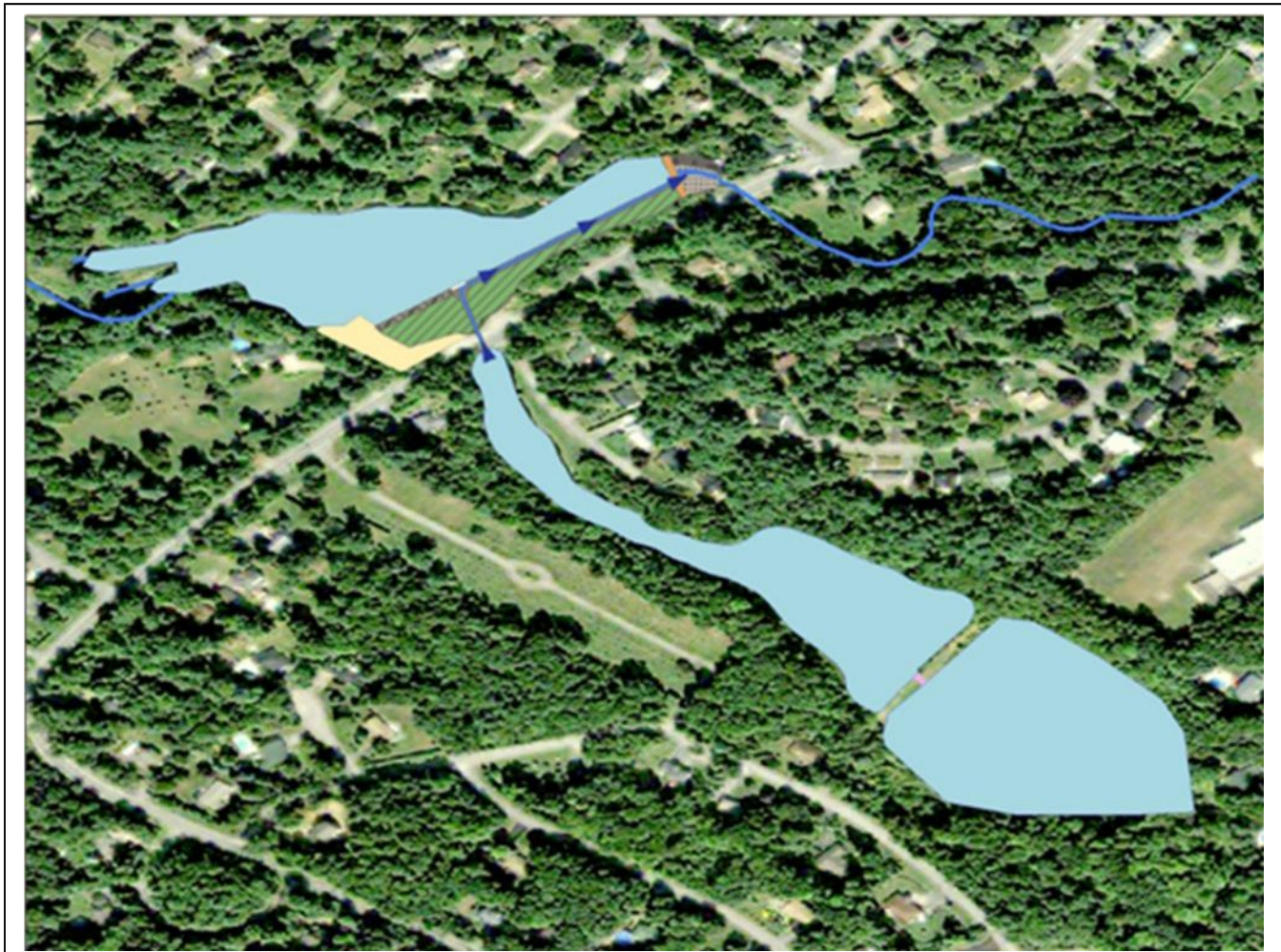
Figure 8b. The lower reach of Black Creek as an auxiliary retention basin. During major floods the town could open the overflow gate in the side of the Black Creek culvert to let water drain from the lake to reduce the risk of the dam failing. Lake water would then flow through the Black Creek culvert into the Viviry below the dam and also spill upstream in Black Creek to flood the marshy areas associated with the Driscoll-Naylor Bird Sanctuary. Periodic flooding would be advantageous to the marsh vegetation and provide temporary flood retention capacity without risk to residential properties.
